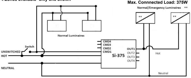
Note: Multiple zone wiring can be duplicated - Only One zone is shown.
