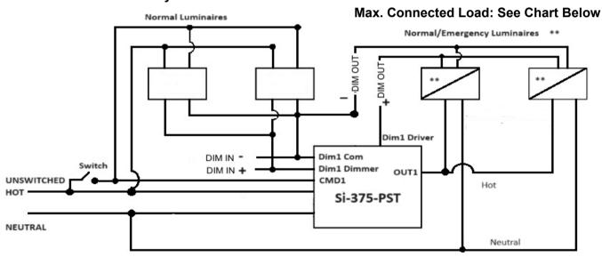
Note: Multiple zone wiring can be duplicated - Only One zone is shown.
